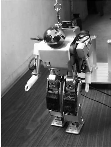
Figure 7: Hardware model of biped robot, HOAP-1 (Fujitsu Automation)
