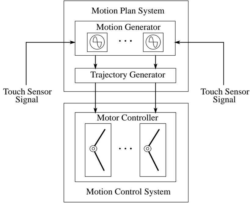
Figure 3: Architecture of Locomotion Control System
