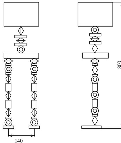
Figure 1: Schematic model of biped robot (1)
