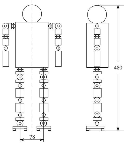
Figure 2: Schematic model of biped robot (2)
