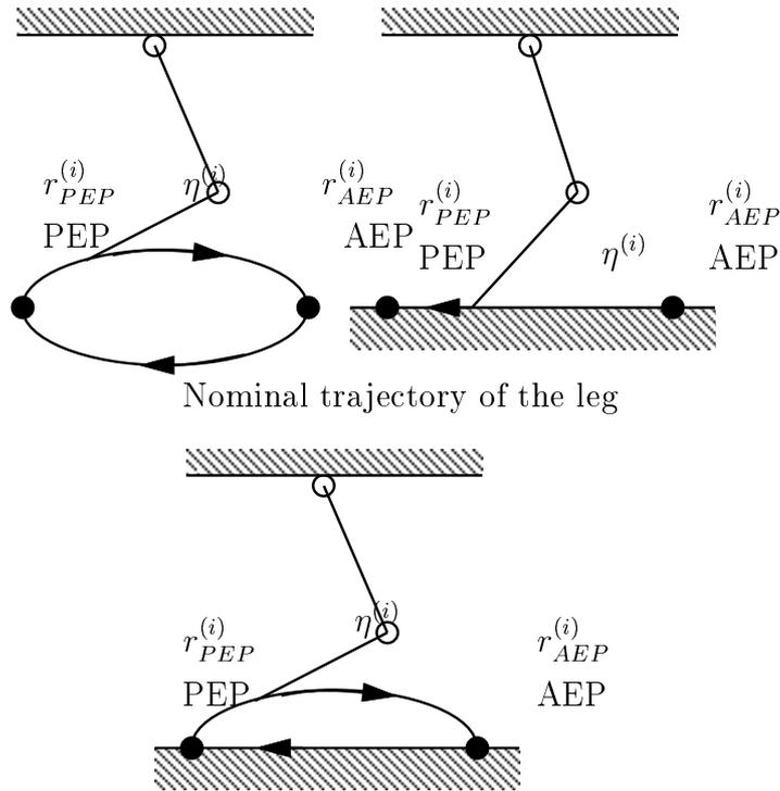
Figure 5: Trajectory of the leg
