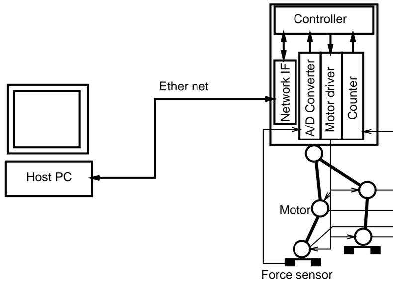
Figure 10: Block diagram of the hardware model
