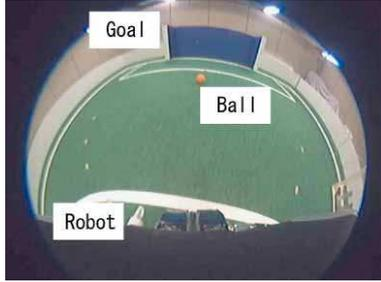
**Fig. 13.** Robot's view (CCD camera image through fish-lens)
