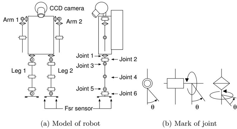
**Fig. 1.** A model of biped locomotion robot
