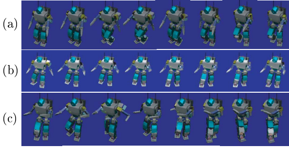
Fig.3 Generated motions on a humanoid robot (a):walk (b):walk+kick (c):kick
