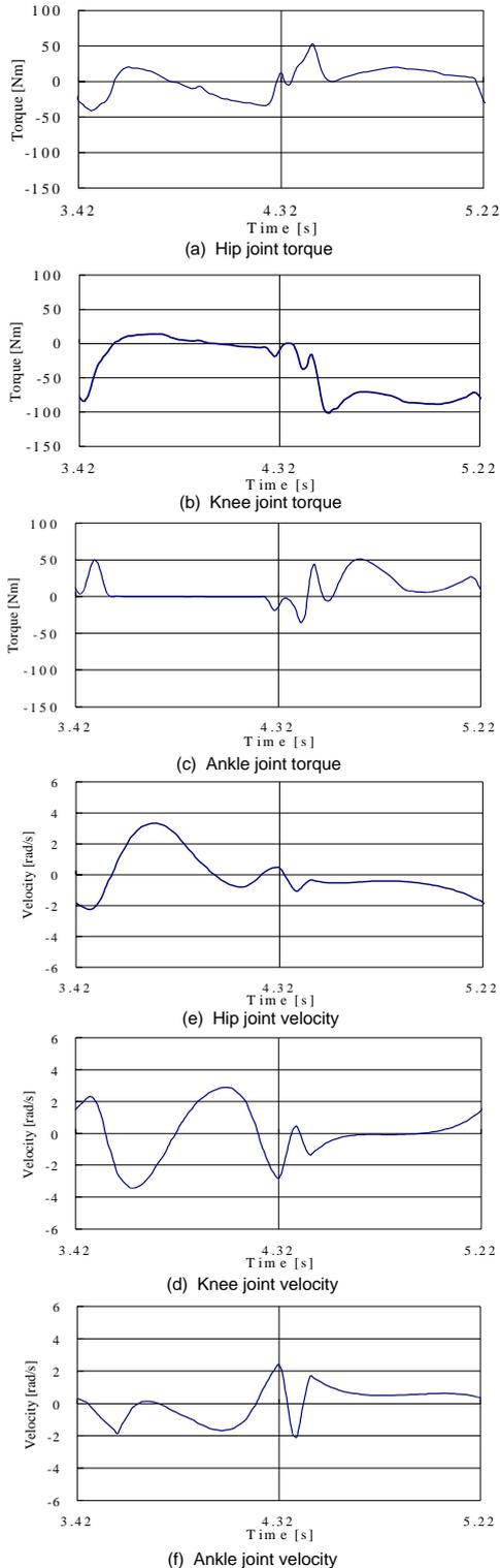
Fig. 8: Required actuator specification
