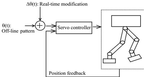
Fig. 4: Structure of balance controller
