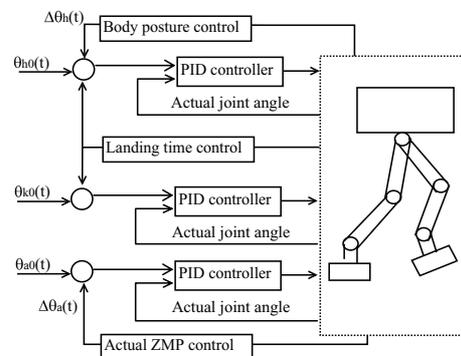
Fig. 7: Block diagram of balance control
