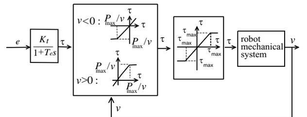
Fig. 2: Actuator simulator model
