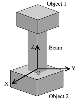
Fig. 3: Force simulator model
