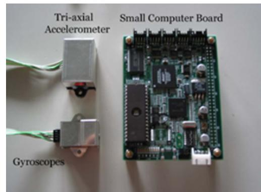
Fig.1 Sensor and Processing Board
