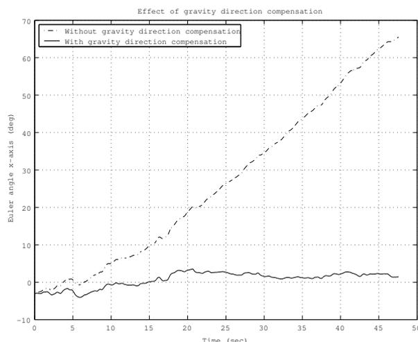
Fig.2 Effect of Gravity Direction Compensation
