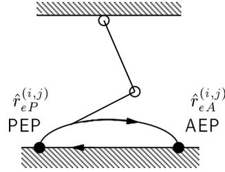
Fig. 3: Nominal trajectory of the tip of the leg
