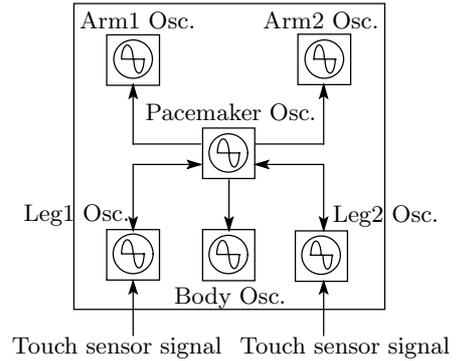
**Figure 3:** Motion generator system
