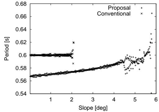
Figure 7: Period of locomotion (In the case of the change of the slope angle)
