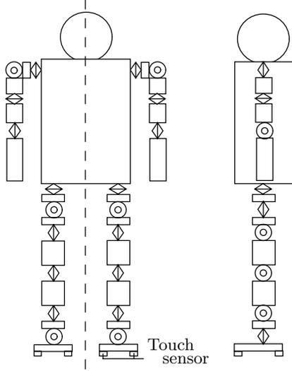
**Figure 1:** Schematic model of biped locomotion robot
