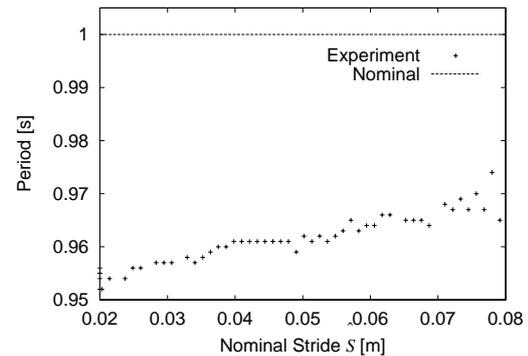
**Figure 9:** Period of locomotion (In the case of the change of the locomotion speed)
