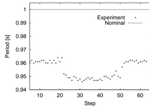
**Figure 10:** Period of locomotion (In the case of the change of the slope angle)
