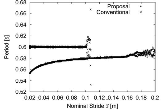
Figure 6: Period of locomotion (In the case of the change of the locomotion speed)
