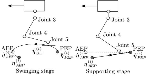
Figure 5: Modified trajectory of the leg
