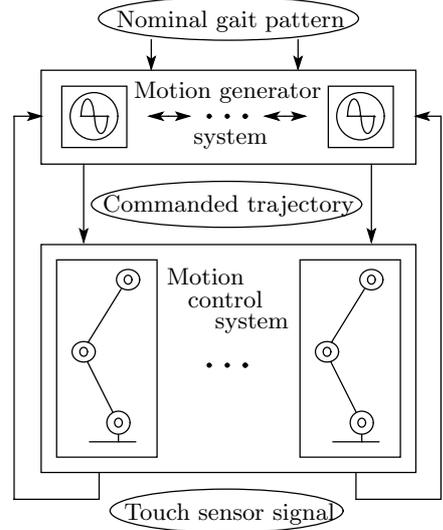
**Figure 2:** Locomotion control system
