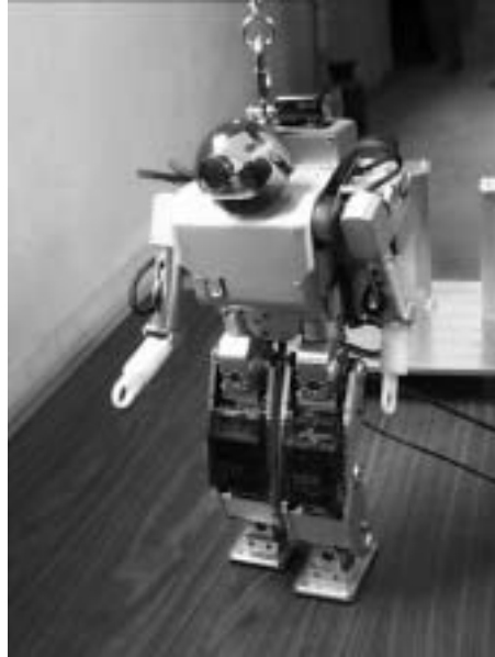
Fig.11. Hardware model of biped robot, HOAP-1 (Fujitsu)
