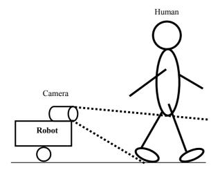
Fig 1 . Robot measures human's walking pitch
